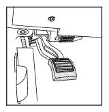
The parking brake pedal is located to the left of the regular brake pedal, near the driver's door.
